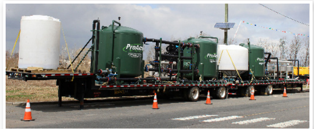
2000 gallon per minute water treatment system
